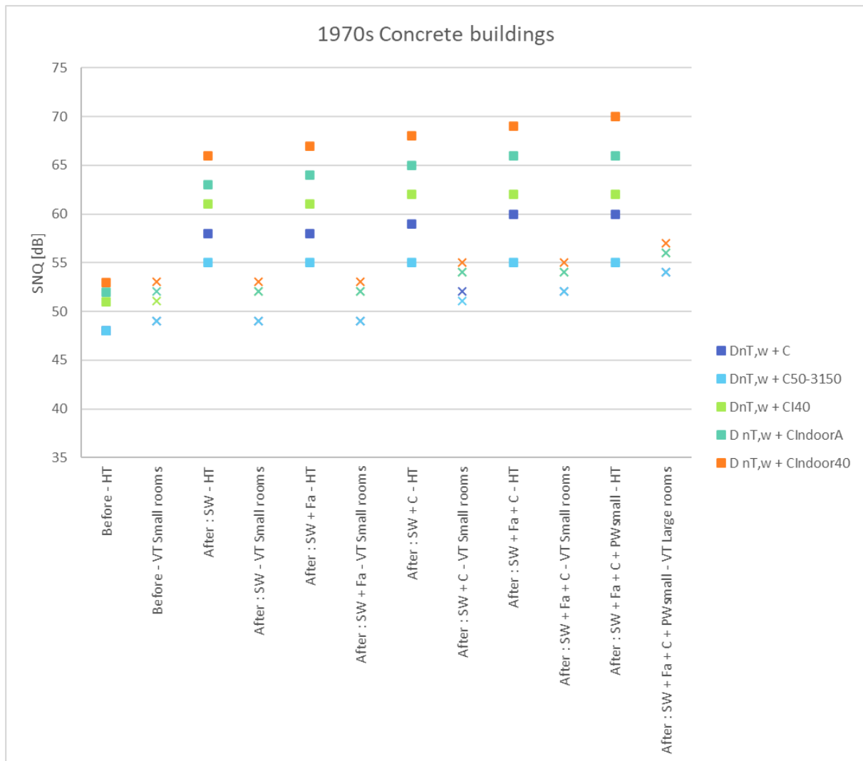
Figure 5.2.1: 1970s building with concrete based separating wall – Step-by-step building improvement – Airborne sound insulation performance in dB.
